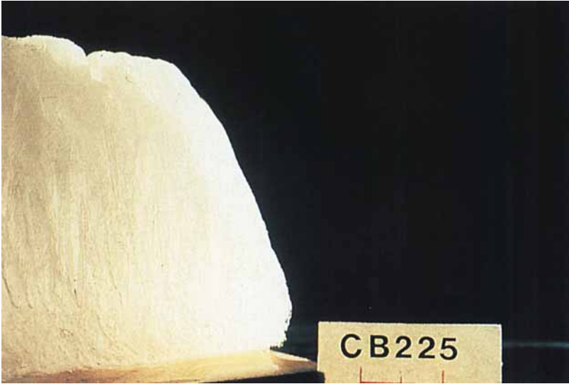
FIGURE 7. A photograph taken in the vertical plane which reveals the form of the resulting product obtained by cooling an aqueous solution of \text{NaNO}_3 to form ice. Note the uneven upper surface and the almost vertical crevices in the solid ice which contain compositionally enriched fluid. The horizontal scale beneath CB225 is 2 cm long. Conditions of the experiment: T_B = -16.5^\circ\text{C} , T = 14.7^\circ\text{C} , C = 14 wt% \text{NaNO}_3 .
