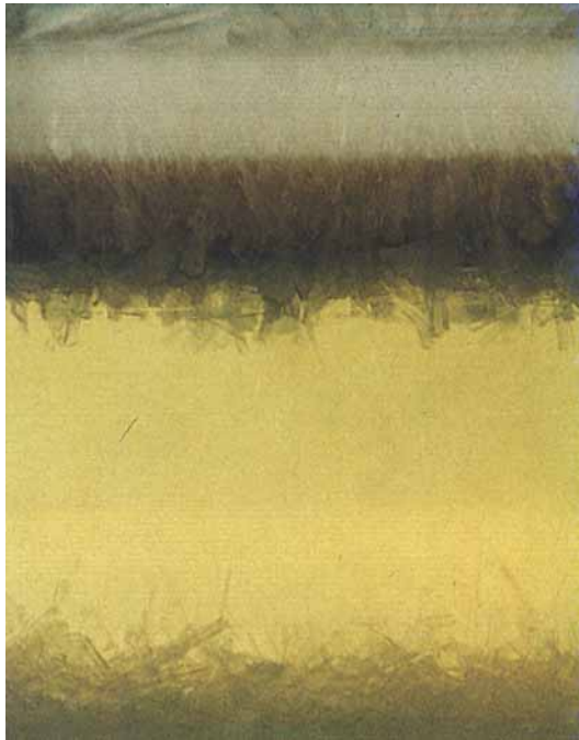
FIGURE 14. A photograph taken during an experiment in which an aqueous solution of \text{Na}_2\text{SO}_4 was cooled from above to form a composite layer next to the roof of the tank, a mushy layer below this and a layer of faceted \text{Na}_2\text{SO}_4 \cdot 10\text{H}_2\text{O} crystals at the base. The experimental conditions were: C_0 = 16 wt% \text{Na}_2\text{SO}_4 , T_0 = 30.5^\circ\text{C} , T_B = -17^\circ\text{C} , and H = 18.8 cm.
